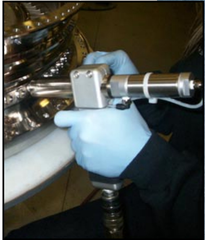
HRP-1 installing snap rings in a jet engine at GE Aviation, Durham, NC
